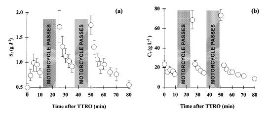
Figure 5. (a) Normalized instantaneous sediment output ( $S_t$ ) and (b) instantaneous sediment concentration ( $C_t$ ) for the pre-pass and two post-pass phases of the MOTORCYCLE simulations. Rainfall was stopped for 15 min to make the motorcycle passes. Each phase time series begins when runoff was generated. Values are means  $\pm$  one standard error
