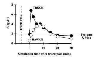
Figure 9. Comparison of post-pass instantaneous sediment transport ( $S_t$ ) for the TRUCK simulations (reported herein) and a previous study in Hawaii (A. D. Ziegler, unpublished data). In both experiments, post-pass values decrease to approximately the pre-pass maximum value after about 20 min (33 and 40 mm of rainfall for the Hawaii and Thailand simulation, respectively)
