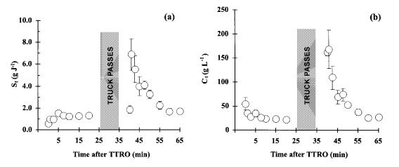
Figure 6. (a) Normalized instantaneous sediment output ( $S_t$ ) and (b) instantaneous sediment concentration ( $C_t$ ) for the pre-pass and post-pass phases of the TRUCK simulations. Rainfall was stopped for 10 min to make the truck passes. Each phase time series begins when runoff was generated. Values are means  $\pm$  one standard error
