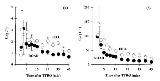
Figure 4. (a) Normalized instantaneous sediment output ( $S_t$ ) and (b) instantaneous sediment concentration ( $C_t$ ) for the FILL and ROAD simulations. Values are means  $\pm$  one standard error
