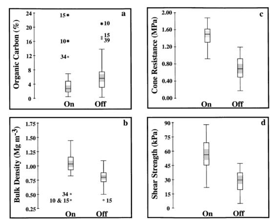
Figure 2. Selected side-by-side box plots of on- and off-trail soil variables: (a) organic carbon (*OC*); (b) bulk density ( $\rho_B$ ); (c) penetration resistance (*PR*); and (d) vane shear strength ( $\tau_{\nu}$ ). Note the numbers associated with the outliers represent sample site locations.
