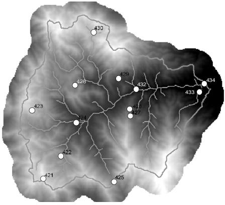
**Fig. 2** The location of hydro-meteorological measurement instruments in the 74.16 km<sup>2</sup> Mae Sa Catchment. Streamflow and turbidity has been monitored at one location (434); energy flux variables for estimating evapotranspiration at three locations (421, 429, 433); soil moisture at six locations (421, 423, 425, 428, 429, 433); and rainfall at all locations but Stations 427 and 434.
