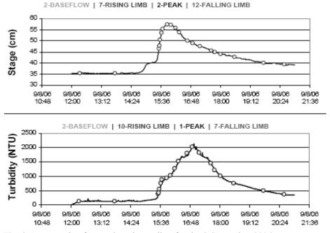
**Fig. 3** An example of storm-based sampling for the 8 September 2006 event. Dots represent sampling times with respect to recorded stage or turbidity.
