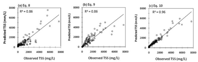
Fig. 5 Comparison of observed total suspended solids (TSS) concentrations with those predicted via regression using (a) discharge; (b) turbidity, and (c) discharge and turbidity.
