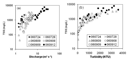
Fig. 4 Observed total suspended solids (TSS) concentrations during the six storms and their corresponding discharge (a) and turbidity (b) values.
