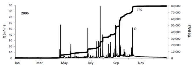
Fig. 6 Mean hourly discharge (Q) and cumulative TSS load (74 032 t) for the year 2006.
